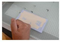
Now you have poured in the casting mix, you can just tap or thump on the table or platform and this will help the wet mix flow into any gaps which ensures you do not have to overfill the moulds and there is less waste when levelling off
